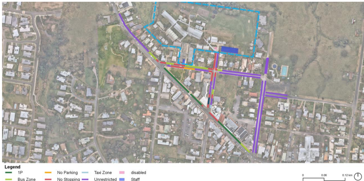
Figure 3-3 On-street parking restrictions
